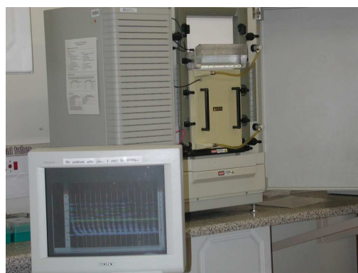
Figure 2.3 (b) The ABI Prism® 377 Automated DNA Sequencer with an example of a gel image
